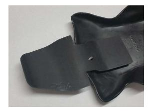
First, slide the Obie Link Guard in between the skid plate and the frame (with the engraved side up on the right side of the bike and the curled-up end by the shock). It may be necessary to grind the holes out on your skid plate (as the arrow shows) so that the mounting holes in your skid plate will line up with the mounting tabs on the frame. Always mount the Obie Link Guard between the frame and your skid plate for a smooth transition from skid plate to link guard.
