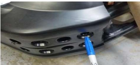
Next put the skid plate on without the metal mounting brackets. Mark the engine so you know where to mount the metal mount/tabs
