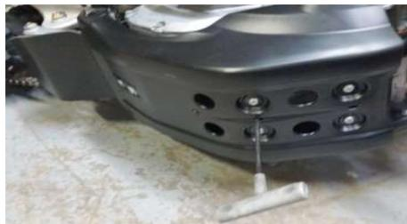
Start all allen bolts through the skid plate then tighten the bolt in the middle of each mounting plate.
