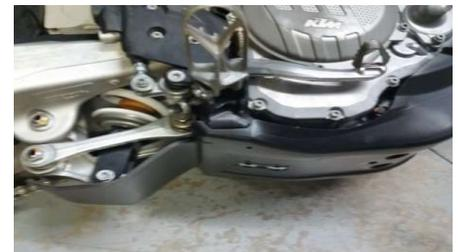
The NEW 2016 4-stroke chassis makes the linkage hang lower than previous model years
