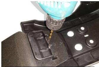
Drill two 7/32 holes on each side of hook
