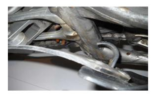
Most Plastic brand skid plates have a hook that goes over the bottom frame for quick and easy on/off installation. First, slide the Obie Link Guard over the hook (with the engraved side up on the right side of the bike & curled up end by the shock) and push the skid plate onto the bottom cross frame (it takes more force the first several times). Always mount the Obie Link Guard between the frame and your skid plate for a smooth transition from skid plate to link guard.
