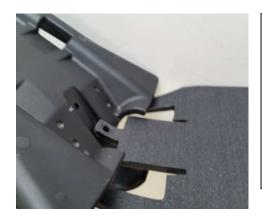
After the Link Guard is installed the skid plate will be farther back making it harder to insert the 6mm bolts.
