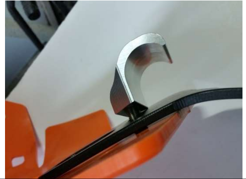
Ready to Install: Leave the bolts loose until you push the hook over the cross tube. All 2-stroke and 450 F only
