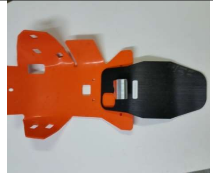
Ready to Install: Leave the bolts loose until you push the hook over the cross tube. All 2-stroke and 450 F only
