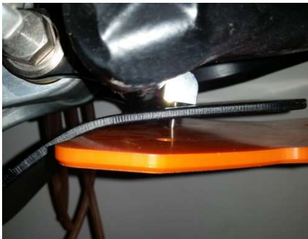
Obie Hold Aluminum Bracket (cut out for drain plug, notch for center case 250-350F) 2 ea 6mm x 25 mm Flat Socket Bolts supplied
