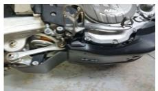
The NEW 2016 4-stroke chassis makes the linkage hang lower than previous model years
