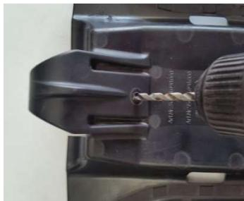
Drill one 3/16 or 5mm hole,  $\frac{1}{4}$  inch down from center rib of the
