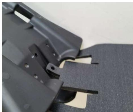
After the Link Guard is installed the skid plate will be farther back making it harder to insert the 6mm bolts. Grind / file the top part of the aluminum hole is recommended for a stronger fitment.
